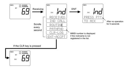
If the CLR key is pressed, the alarm is turned off, the displays are cleared, and the received contents are stored in the Log File. The radio then reverts to the operation mode before receiving the Individual Call.
